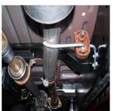
TO REMOVE YOUR STOCK EXHAUST, REMOVE IT FROM THE CLAMP LOCATED JUST IN FRONT OF THE MUFFLER REMOVE HANGERS FROM RUBBER GROMMETS BY PULLING EXHAUST TOWARDS THE REAR OF THE VEHICLE, USE WD-40 TO AID IN REMOVAL, LEAVE GROMMETS IN PLACE.
